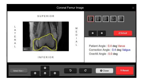
Select size will have drop selection of implant ( size 1 to 8 ). Each arrow button will move implant positioning ( left, right, up, and down ) Rotate arrow will rotate the implant by 3 degrees.
